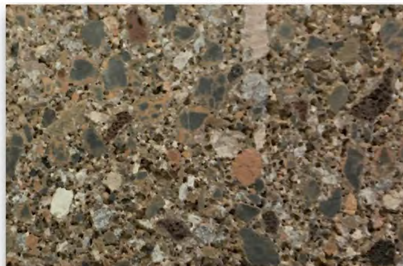
PC-3 : PRE-CAST CONC. PANEL WITH CMU 8 X 16 REVEAL JOINT - GROUND FACE TEXTURE MATCH BEST BLOCK # 329 SEQUOIA
