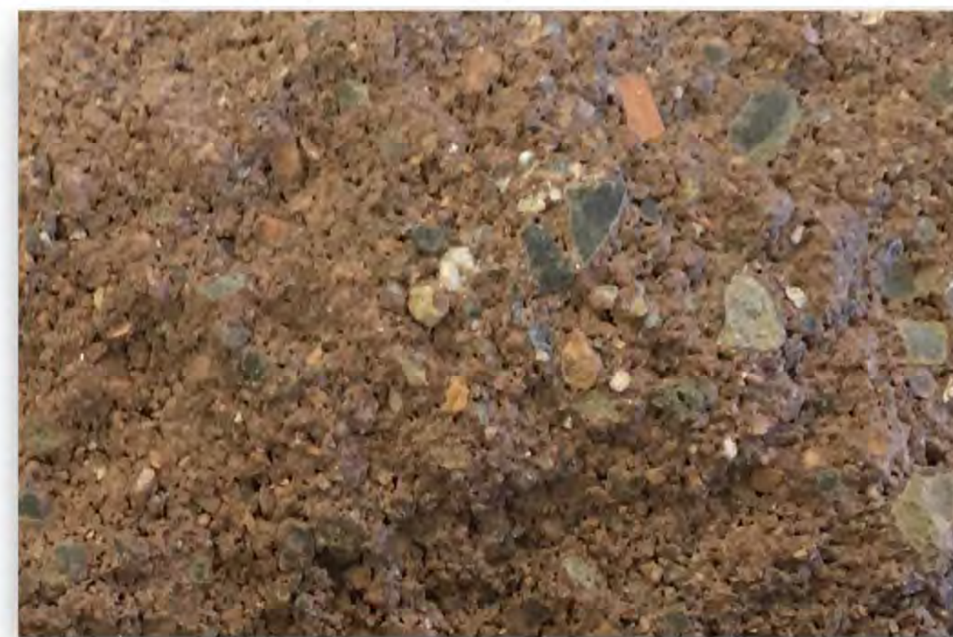
PC-1 : PRE-CAST CONC. PANEL WITH CMU 8 X 16 REVEAL JOINT - SPLIT FACE TEXTURE MATCH BEST BLOCK # 136 MEADOWS
