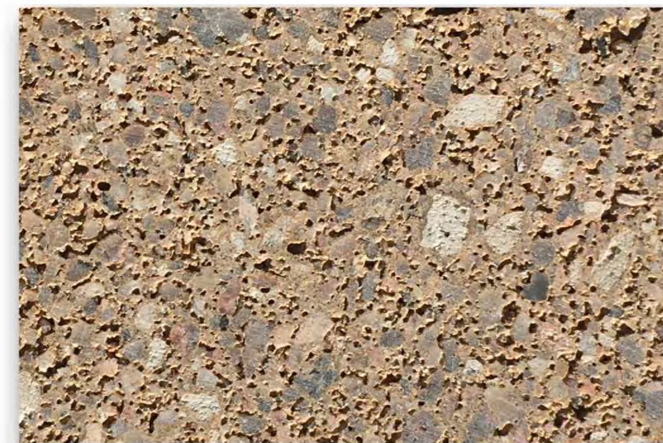
PC-4 : PRE-CAST CONC. PANEL WITH CMU 8 X 8 REVEAL JOINT - GROUND FACE TEXTURE MATCH BEST BLOCK #5447
