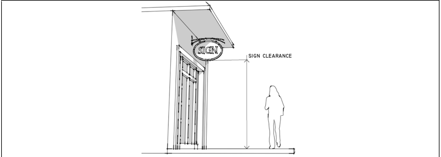
Figure 3.3.11-2 Sign Clearance Measurement
