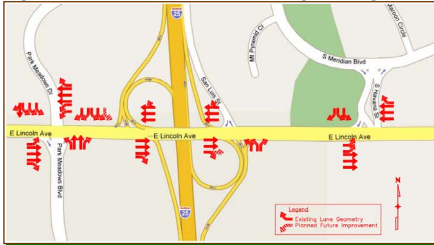
Figure 3 - Lincoln Avenue Interchange Configuration
